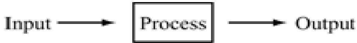
Fig. 1 Block diagram of an open loop control system
