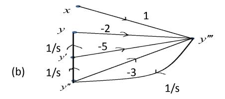
Step 4: Reverse the sign of a branch connecting y''' to y'', with condition no change in T/F fn.
