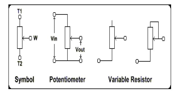
Potentiometers comprise a resistive element, a sliding contact (wiper) that moves along the element, making good electrical contact with one part of it, electrical terminals at each end of the element, a mechanism that moves the wiper from one end to the other, and a housing containing the element and wiper.
