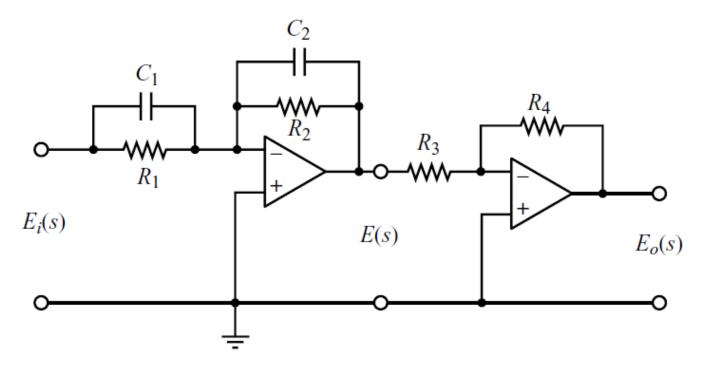
$\frac{E_o(s)}{E_i(s)} = \frac{R_2 R_4}{R_1 R_3} \frac{R_1 C_1 s + 1}{R_2 C_2 s + 1}$
