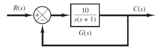
It is desired to design an Electronic lead compensator G<sub>c</sub>(s) so that the dominant closed poles have the damping ratio
