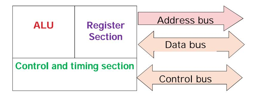
Block diagram of a microprocessor
