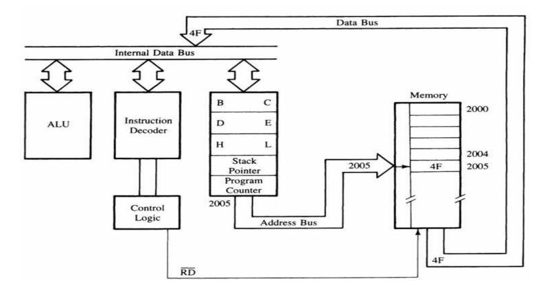
Moving data form memory to MPU using instruction **MOV C**, **A** (code machine 4FH = 0100 1111)
