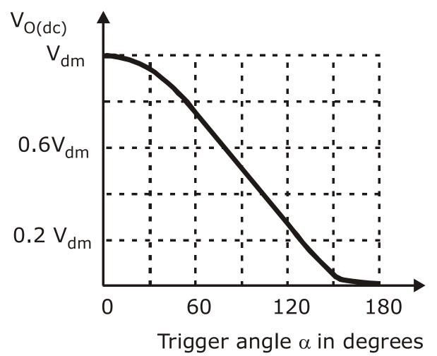
Normalizing the dc output voltage with respect to  $V_{dm}$ , the Normalized output voltage
