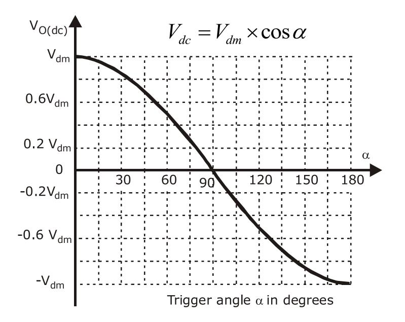
By varying the trigger angle we can vary the output dc voltage across the load. Hence we can control the dc output power flow to the load. For trigger angle  $\alpha$ , 0 to 90<sup>°</sup> (*i.e.*,  $0 \le \alpha \le 90^{\circ}$ );  $\cos \alpha$  is positive and hence  $V_{dc}$  is positive  $V_{dc}$  &  $I_{dc}$  are positive;  $P_{dc} = (V_{dc} \times I_{dc})$  is positive Converter operates as a Controlled Rectifier. Power flow is from the ac source to the load.
