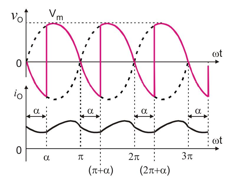
$$V_{O(dc)} = V_{dc} = \frac{1}{\pi} \int_{\omega t = \alpha}^{(\pi + \alpha)} v_O d(\omega t)$$
