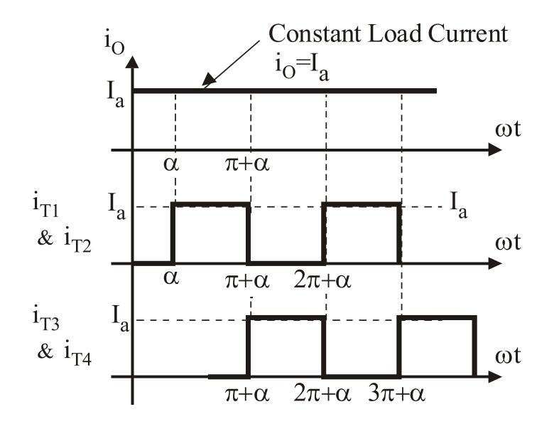
To Derive An Expression For The Average DC Output Voltage of a Single Phase Full Converter assuming Continuous & Constant Load Current The average dc output voltage can be determined by using the expression
