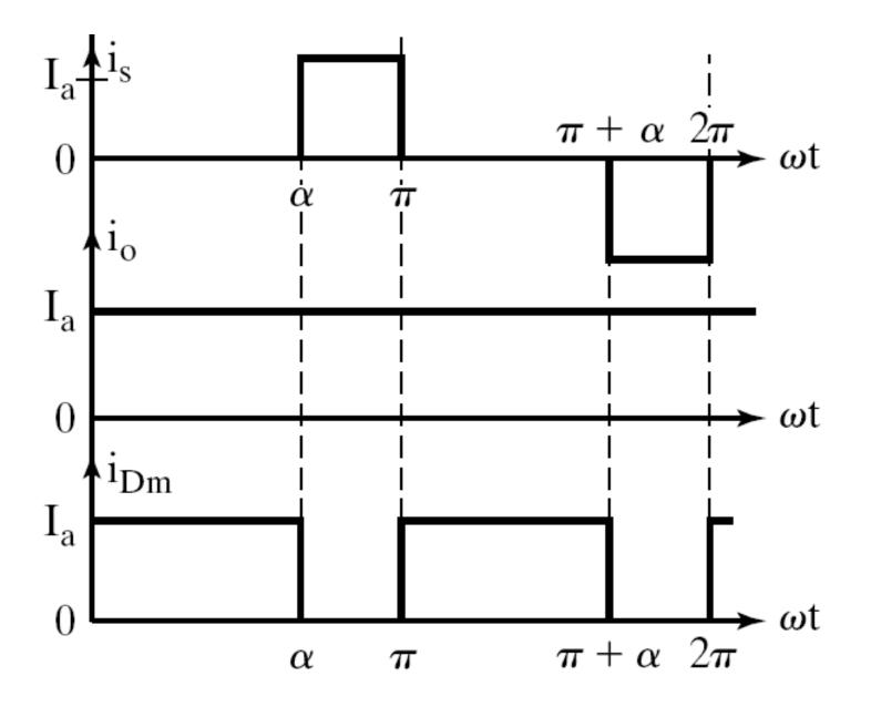
Thyristor  $T_1 \& D_1$  conduct from  $\omega t = \alpha to \pi$ Thyristor  $T_2 \& D_2$  conduct from  $\omega t = (\pi + \alpha) to 2\pi$ FWD conducts during  $\omega t = 0$  to  $\alpha$ ,  $\pi$  to  $(\pi + \alpha), \dots$
