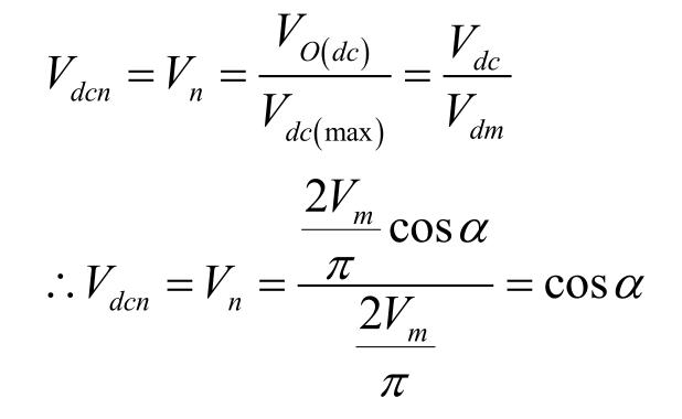
By plotting V<sub>O(dc)</sub> versus α, we obtain the control characteristic of a single phase full wave fully controlled bridge converter (single phase full converter) for constant & continuous load current operation. To plot the control characteristic of a Single Phase Full Converter for constant & continuous load current operation. We use the equation for the average/ dc output voltage
