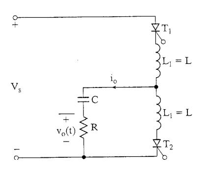
$T_1$  fired, resonant pulse of current flows through the load. The current falls to zero at  $t = t_{1m}$  and  $T_1$  is "self – commutated".
