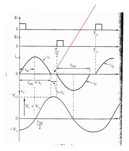
This "off-time" must be longer than the turn-off time of the thyristors,  $t_{\alpha}$ .
