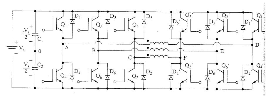
12 transistors, 12 diodes, 3 transformers
