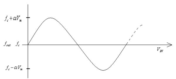
In general, m(t) will be a 'band of signals', *i.e.* it will contain amplitude and frequency variations. Both amplitude and frequency change in m(t) at the input are translated to (just) frequency changes in the FM output signal, *i.e.* the amplitude of the output FM signal is constant.
