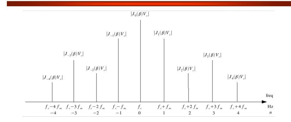
The amplitudes drawn are completely arbitrary, since we have not found any value for  $J_n(\beta)$  – this sketch is only to illustrate the spectrum.
