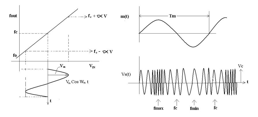
The output frequency varies 'gradually' from  $f_c$  to  $(f_c + \alpha V_m)$ , through  $f_c$  to  $(f_c - \alpha V_m)$  etc.
