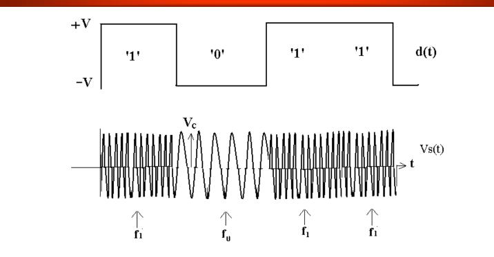
Assuming d(t) = +V for 1's  $f_{OUT} = f_1 = f_c + \alpha V$  for 1's the output 'switches' = -V for 0's  $f_{OUT} = f_0 = f_c - \alpha V$  for 0's between  $f_1$  and  $f_0$ .
