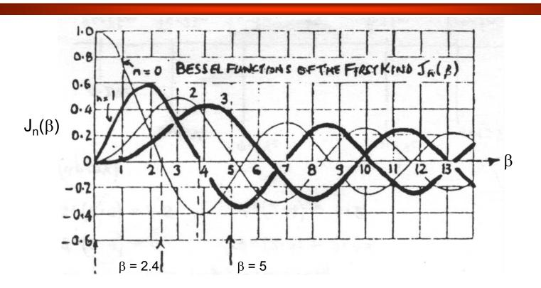
In the series for  $v_s(t)$ , n = 0 is the carrier component, *i.e.*  $V_c J_0(\beta) \cos(\omega_c t)$ , hence the n = 0 curve shows how the component at the carrier frequency,  $f_c$ , varies in amplitude, with modulation index  $\beta$ .
