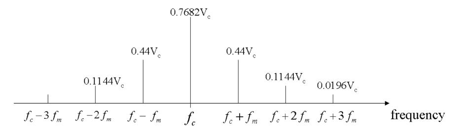
Bandwidth of Significant Spectrum =  $6 f_m$
