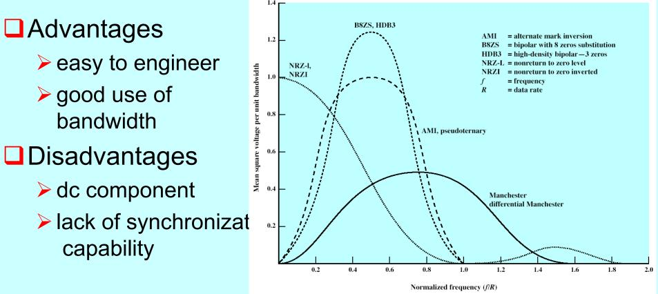
Figure 5.3 Spectral Density of Various Signal Encoding Schemes
