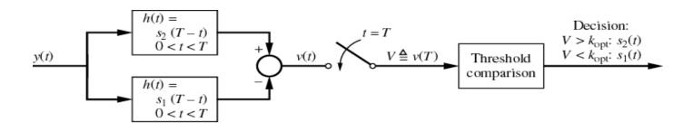
Figure 7-9 Matched filter receiver for binary signaling in white Gaussian noise.
