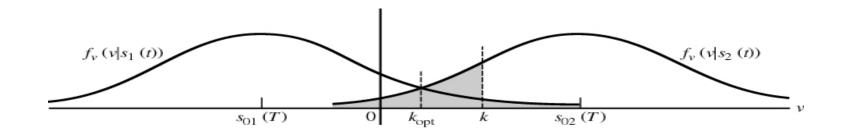
Figure 7-7 Conditional probability density functions of the filter output at time t = T.
