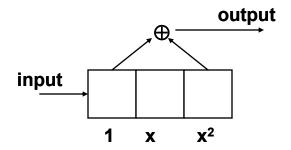
will multiply the input stream by  $x^2+1$  and the second shift register
