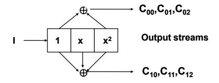
For encoding of convolution codes so called
