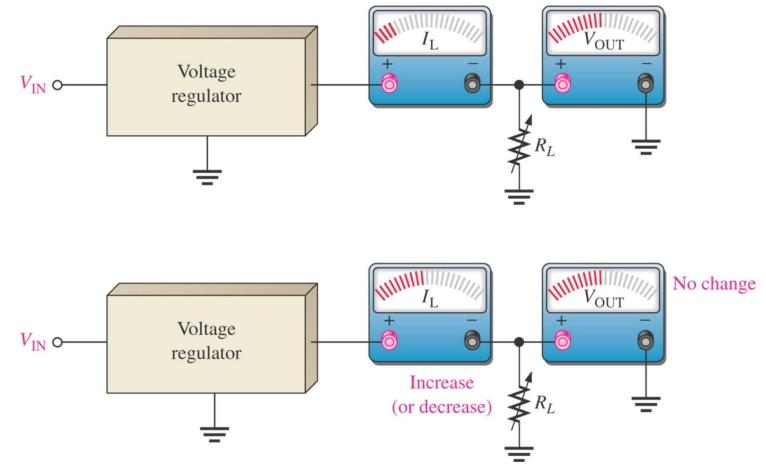
Load regulation: A change in load current (due to a varying  $R_L$ ) has practically no effect on the output voltage of a regulator (within certain limits)
