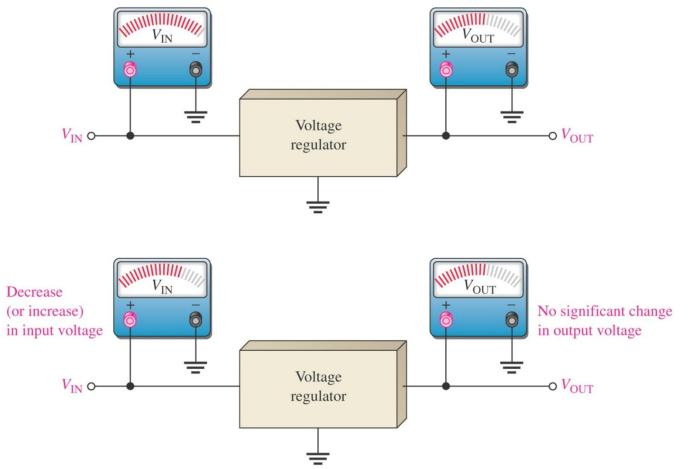
Line regulation: A change in input (line) voltage does not significantly affect the output voltage of a regulator (within certain limits)
