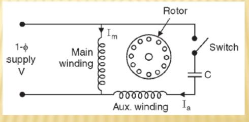
The value of capacitor is so chosen that Ia leads Im by about  $90^{\circ}$ , so that the starting torque is maximum for certain values of Ia and Im. Again, the starting winding is opened by the centrifugal switch when the motor attains about 75% of synchronous speed. The motor then operates as a single – phase induction motor and continues to accelerate till it reaches the normal speed.
