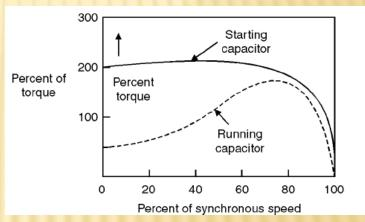
Theoretically, optimum starting and running performance can be achieved by having two capacitors. The starting capacitor is larger in value and is of the ac electrolytic type. The running capacitor permanently connected in series with the starting winding, is of smaller value and is of the paper oil type. Typical values of these capacitors for a 0.5 hp are Cs =300 F, Cr =40 F. The typical torque – speed characteristic is shown in fig.
