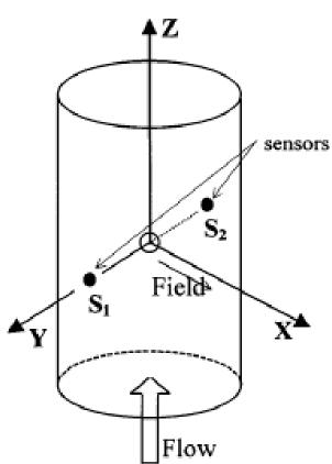
The velocity of the conductor is proportional to the mean flow velocity of the liquid.
