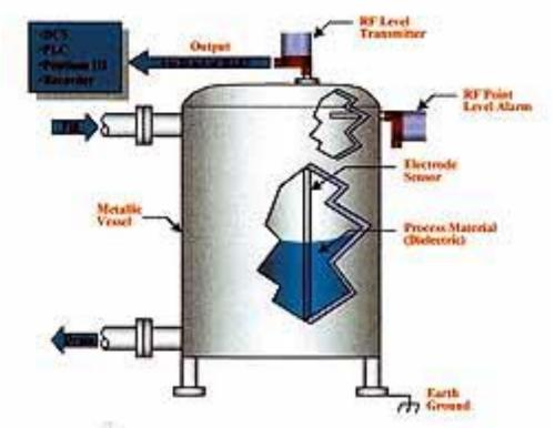
• In the RF capacitance method of liquid level measurement, the electrode sensor connects directly to an RF transmitter outside the tank.
