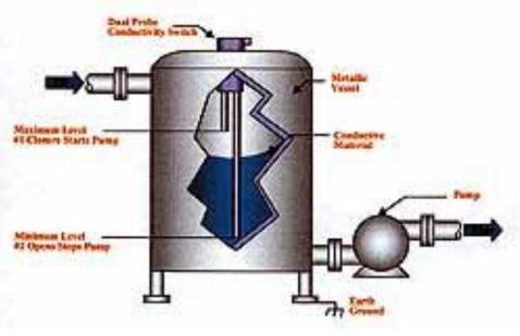
In the conductive type of level measurement, two dual-tip probes detect the maximum and minimum levels in a tank.
