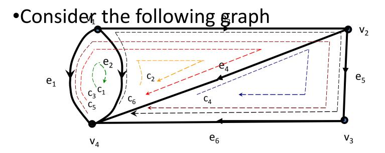
$$\mathbf{B} = \begin{bmatrix} e_1 & e_2 & e_3 & e_4 & e_5 & e_6 \\ \hline -1 & 1 & 0 & 0 & 0 & 0 & c_1 \\ 0 & -1 & 1 & 1 & 0 & 0 & c_2 \\ -1 & 0 & 1 & 1 & 0 & 0 & c_3 \\ 0 & 0 & 0 & -1 & 1 & 1 & c_4 \\ -1 & 0 & 1 & 0 & 1 & 1 & c_5 \\ 0 & -1 & 1 & 0 & 1 & 1 & c_6 \end{bmatrix}$$
