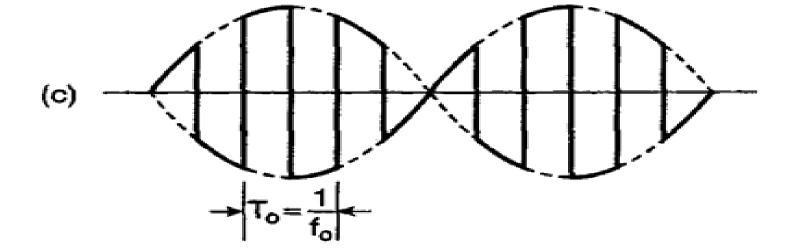
Step-up frequency conversion can be achieved by alternately switching high frequency switching devices (e.g. IGBTs, instead of thyristors) between positive and negative limits at high frequency to generate carrier-frequency modulated output.
