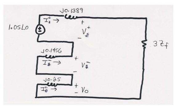
With the sequence networks in series we can solve for the fault currents (assume Z<sub>f</sub>=0)
