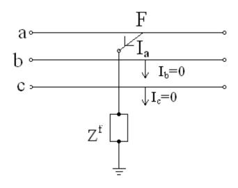
Consider a fault between phase a and ground through an impedance z<sub>f</sub>
