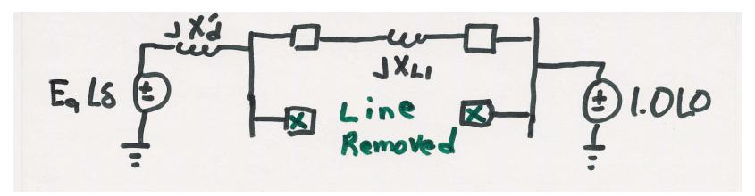
The equivalent system after the fault is then
