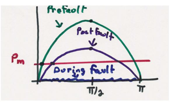
During the disturbance the form of  $P_e(\delta)$  changes, altering the power system dynamics:
