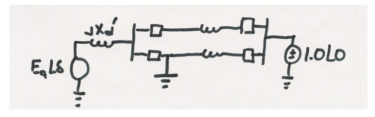
The equivalent system during the fault is then
