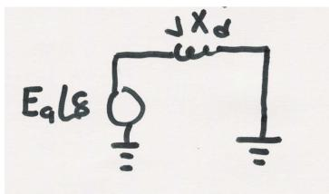
During this fault no power can be transferred from the generator to the system
