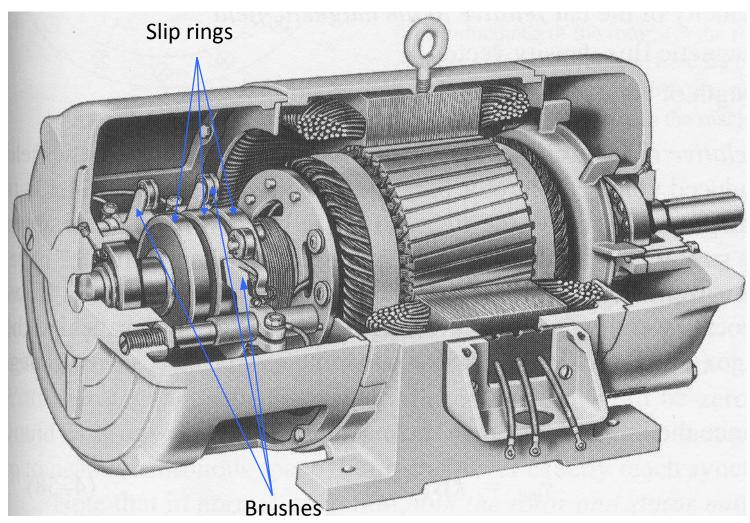
Cutaway in a typical wound-rotor IM.
