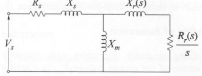
For system studies, the rotor should be represented by a single rotor circuit whose parameters vary as a function of slip, s.
