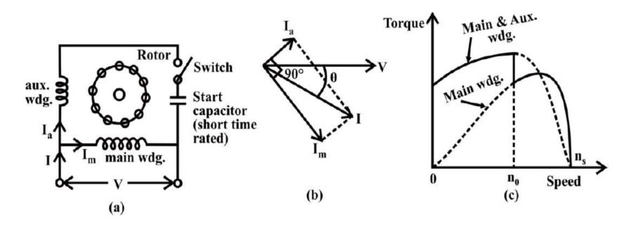
used in applications, such as compressor, conveyor, machine tool drive, refrigeration and air-conditioning equipment, etc.
