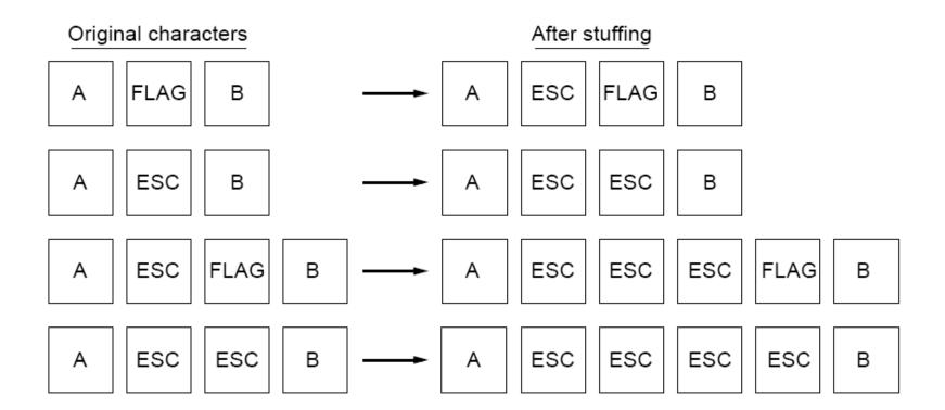
Four examples of byte sequences before and after byte stuffing
