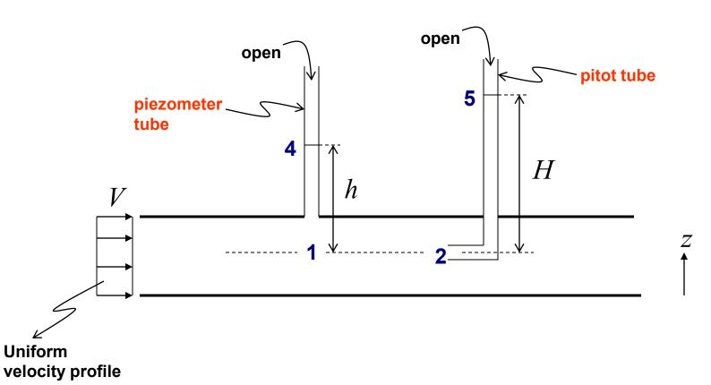
Velocity at point 1 is the velocity of the flow:  $V_1 = V$
