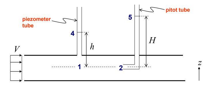
Stagnation pressure is pressure where velocity is zero (at entrance of pitot tube (pt. 2))
