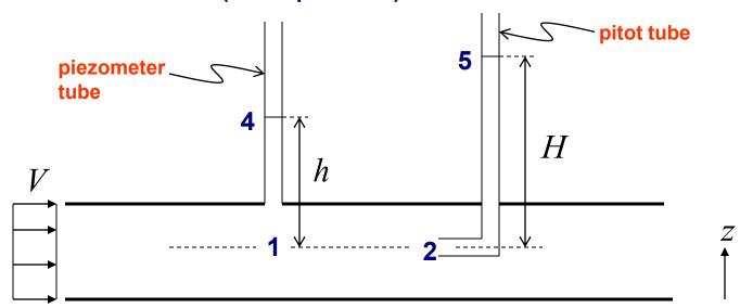
To measure static pressure say at point 1 we use piezometer tube along with  $p + \gamma z = constant$  across straight streamlines between pts. 1 and 4:
