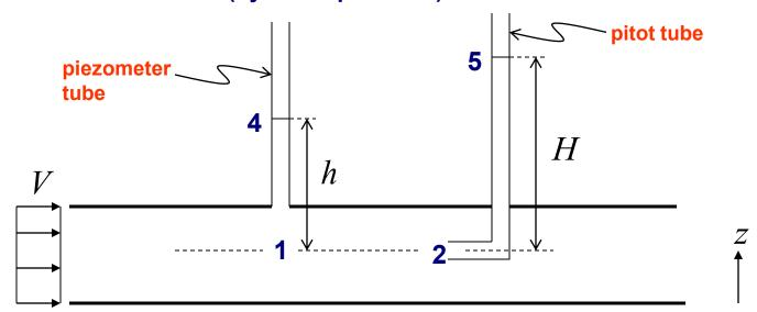
To measure dynamic pressure say at point 1 we use pitot tube along with Bernoulli equation from point 1 to point 5:
