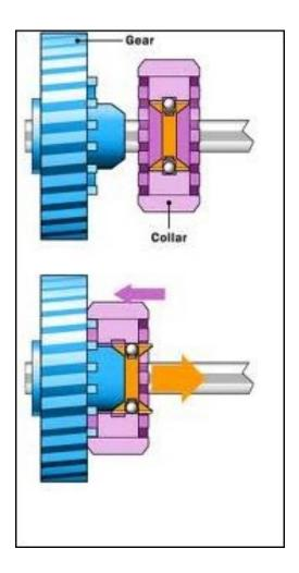
✓ A dog clutch is a type of clutch that couples two rotating shafts or other rotating components not by friction but by interference.
