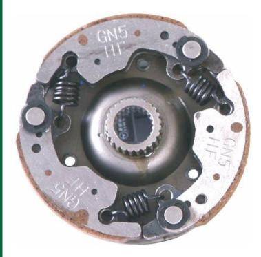
✓ This clutch system employs centrifugal force to automatically engage the clutch when the engine rpm rises above a threshold and to automatically disengage the clutch when the engine rpm falls low enough.
