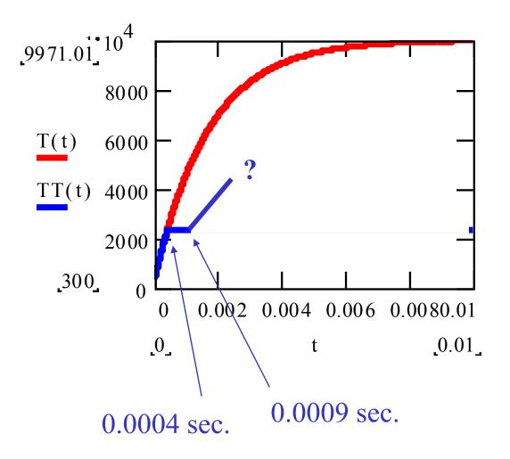
• Temperature of the particle increases exponentially from 300 K to 10000K in a very short time (<0.01 sec.) • It only takes 0.0004 sec. To reach the melting temperature • Therefore, the true temperature variation is described by the blue curve. (why?)
