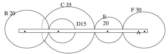
Q-14 In a reverted epicyclic gear train, as shown in figure 4, the arm A carries two gears B and C and compound gear D-E. The gear B meshes with gear E, the gear C meshes with gear D. The number of teeth in gears B, C and D are 75, 30 and 90 respectively. Find the speed and direction of gear C when gear B is fixed and the arm A makes 1000 rpm clockwise.
