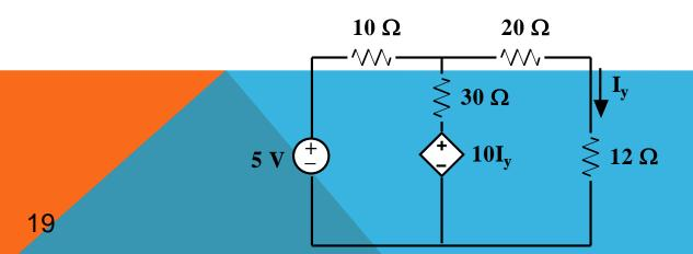
A circuit with a current controlled dependent voltage source.
