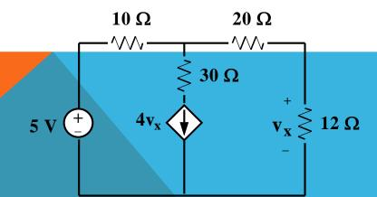
A circuit with a voltage controlled dependent current source
