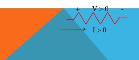
Notice that the voltage is measured across the device
