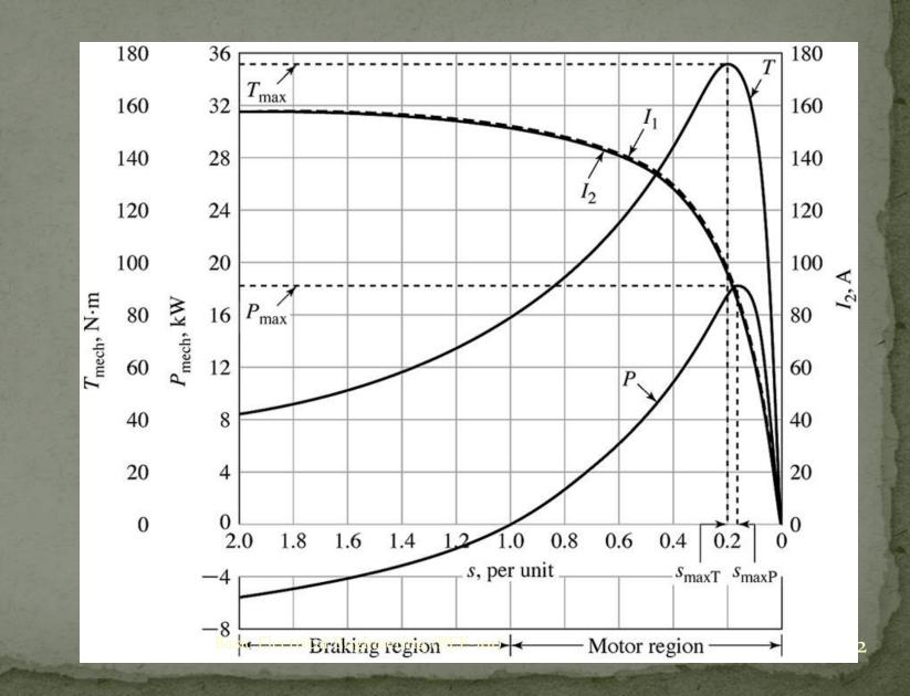
Induction-motor torque-slip curves showing effect of changing rotorcircuit resistance.
