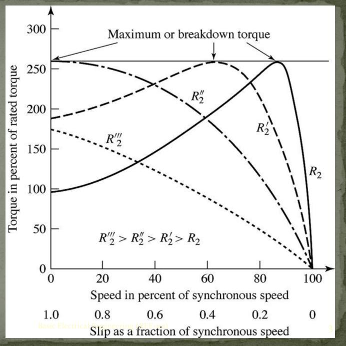
Electromechanical torque vs. speed for the wound-rotor induction motor of Example 6.4 for various values of the rotor resistance  $R_2$ .
