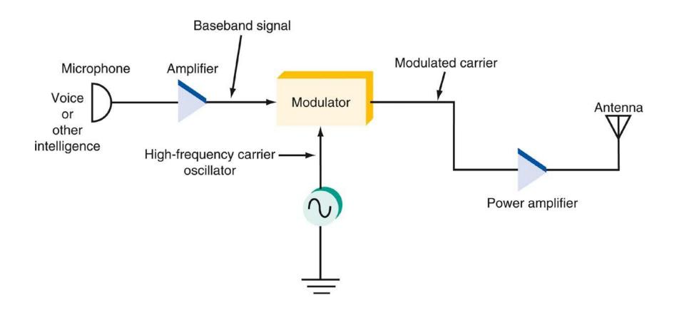
Figure 1: Modulation at the transmitter.
