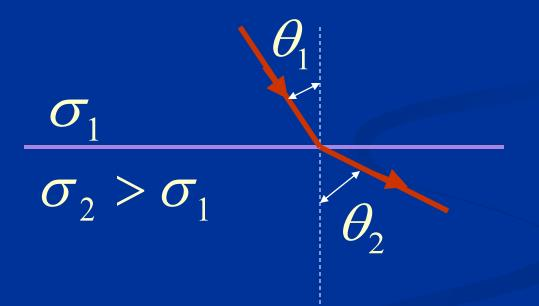
Conductor-Conductor Interface (Cont'd) The angles are related by  $\theta_2 = \tan^{-1} \left( \frac{\sigma_2}{\sigma_1} \tan \theta_1 \right)$
