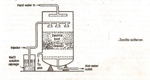
hardness-causing ions  $(Ca^{2+}, Mg^{2+}, etc.)$  are retained by the zeolite as CaZe and MgZe ; while the outgoing water contains sodium salts. Reactions taking place during the softening process are :
