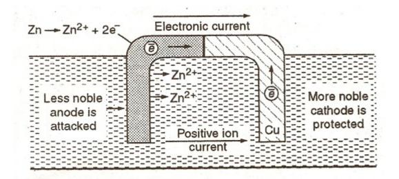
Galvanic corrosion can be minimised by
