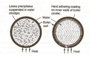
Scale and sludge in boilers.
