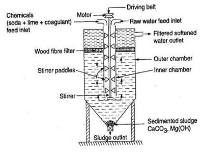
**METHOD:** Raw water and calculated quantities of chemicals (Lime + soda + Coagulants) are fed from the top into the inner vertical circular chamber, fitted with a vertical rotating shat carrying a number of paddles. As the raw water and chemicals flow down, there is a vigorous stirring and continuous mixing, wherebysoftening of water reaches up. The
