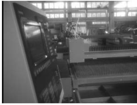
Figure 9. Ytterbium Fiber Laser machine used for drilling in 10 % volume Aluminium-Alumina composite material
