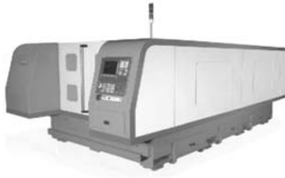
Fig 6, Fiber Laser Machine YLR 2000 used to cut the Al-A1O of volume 10%
