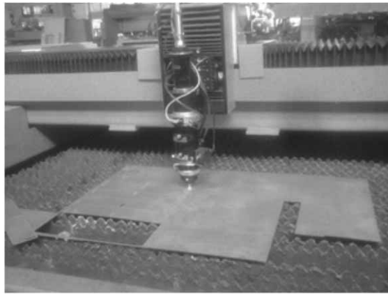
Figure-2 ytterbium laser machining is done on 5 mm thick EN353 steel.
