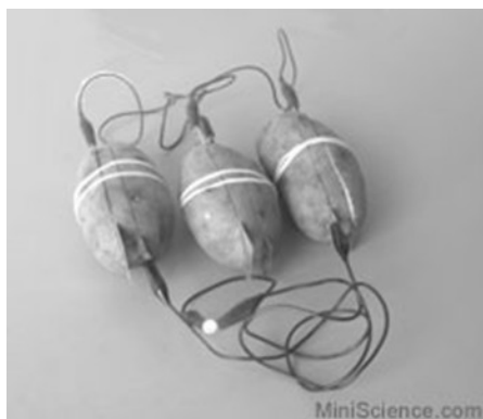
Fig. 4.4 LED/DC Lamp powered by Potatoes
