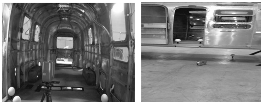
Figure 2: Reference sphere set to receive pulse from laser scanner
