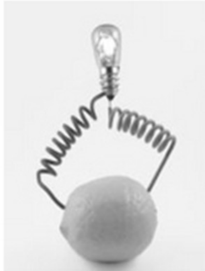
Fig. 4.7 Lemon powered DC Lamp
