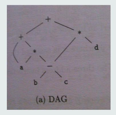
$T_1 = b - c$   $T_2 = a * t_1$   $T_3 = a + t_2$   $T_4 = t_1 * d$  $T_5 = t_3 + t_4$
